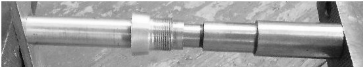
exhaust valve seat installation
