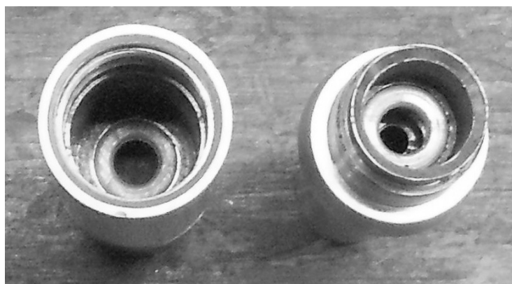
this shows the new seats installed
