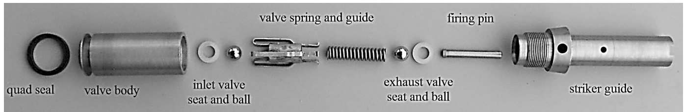
valve unit components
